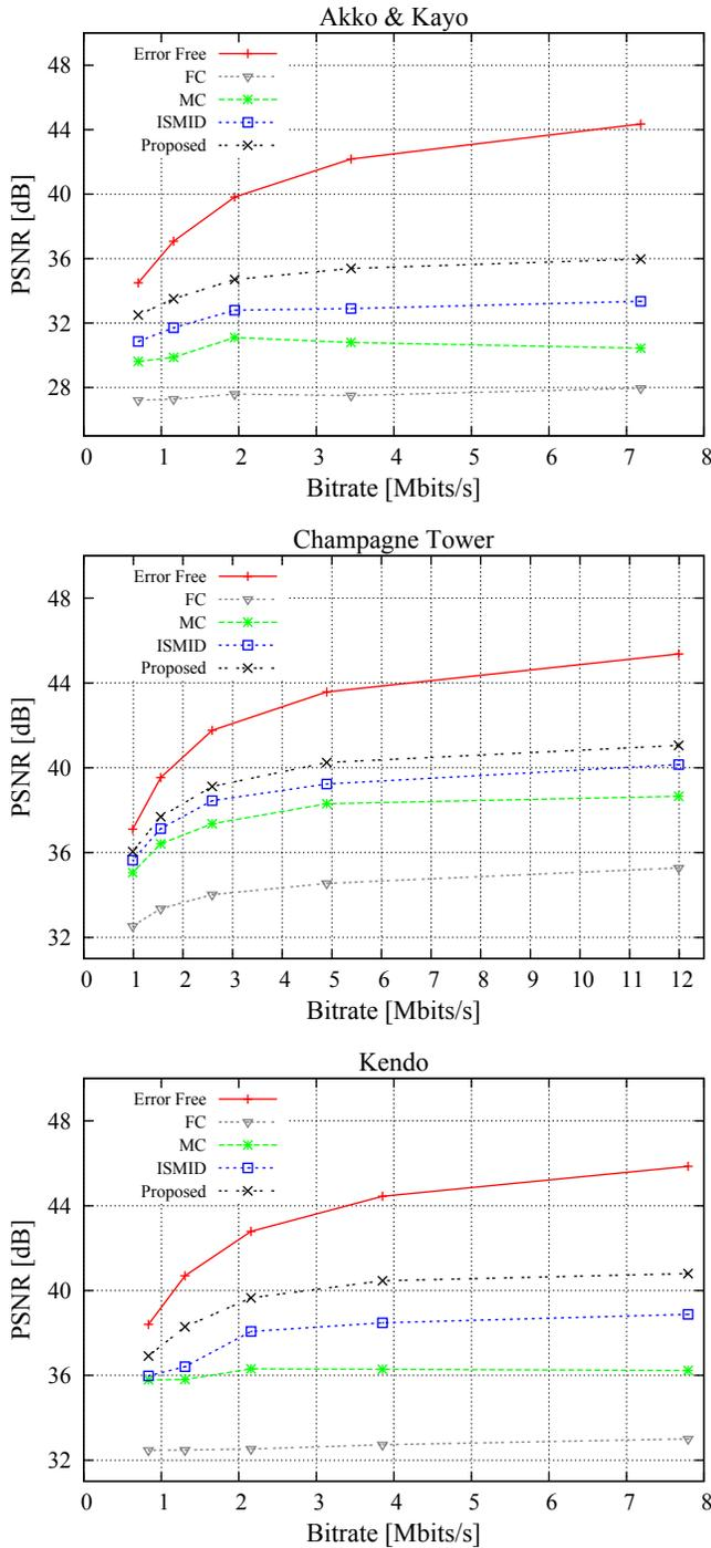
Figure 3: Average quality evaluated with the PSNR under 10% of frame loss.
